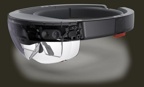
Holographic computer running Windows 10 V1 Announced in 2015, V2 scheduled in 2019 Self-contained, head-worn Multiple sensors, advanced optics, custom chips Displays mixed reality (holograms) Learns about the environment (spatial mapping) Recognizes gestures, voice Cost \$3000 - \$5000 per unit
